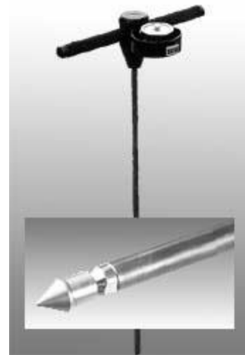
Figure 1. Example of hand held static cone penetrometer. Photo courtesy Durham Geo Corp.
